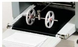
A powered exit conveyor ensures smooth ejection of folded paper.
